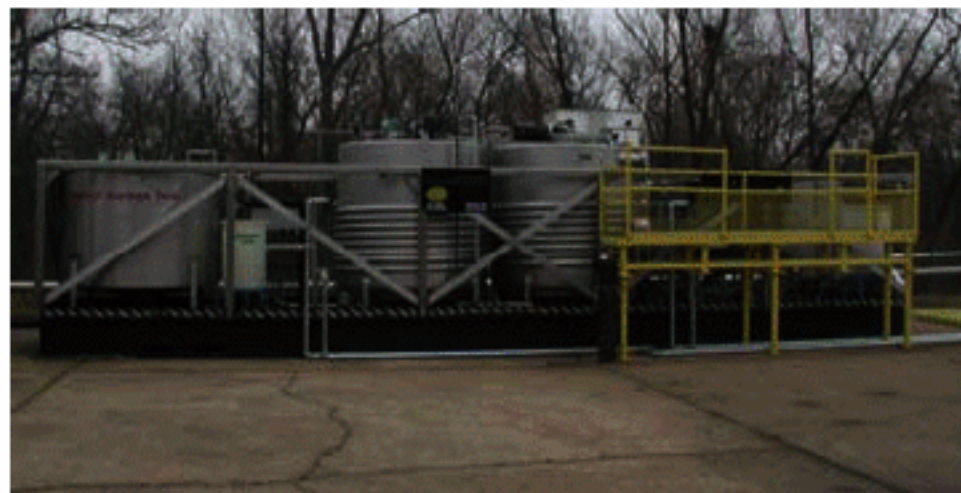
Actodemil® Unit for Safe Destruction and Recycling of Explosives into Fertilizer
