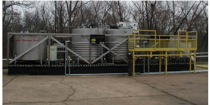
Actodemil® Unit for Safe Destruction and Recycling of Explosives into Fertilizer
